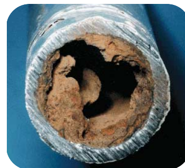
Durapipe superFLO resists the limescale build-up common in most metal pipe materials as shown in the picture above.
